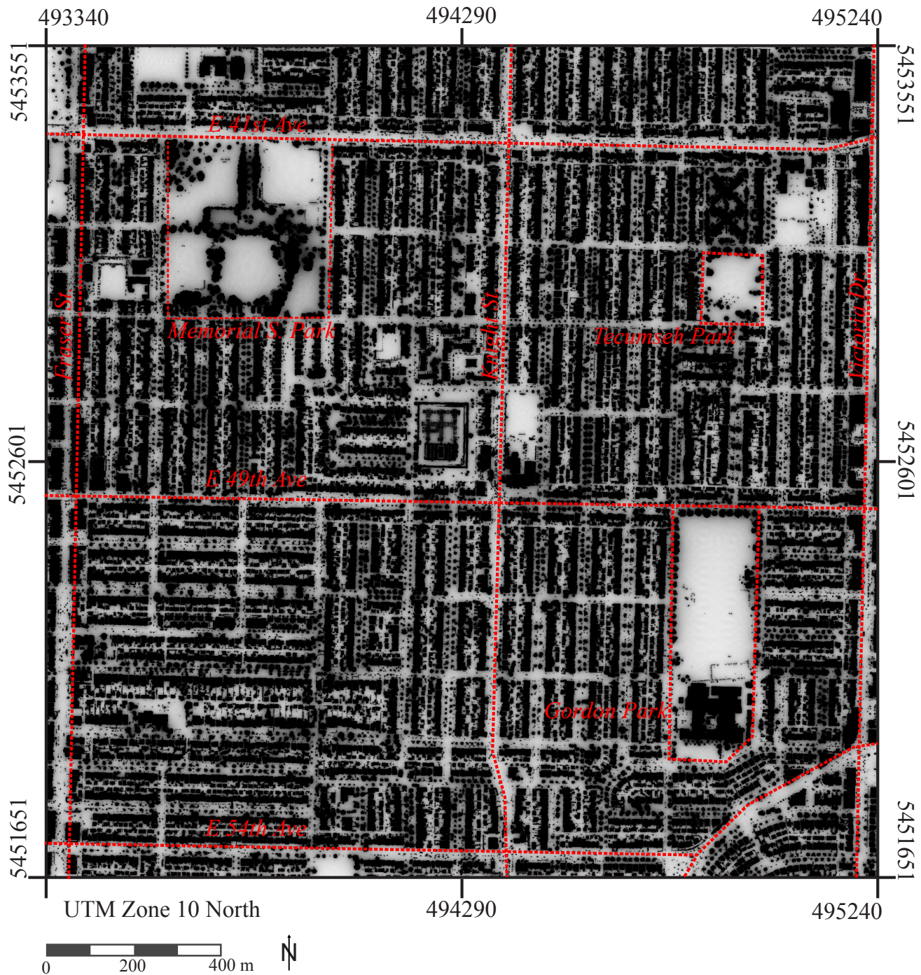
Figure 4 – Map of the sky view factor \psi_{sky} at ground level, from \psi_{sky}=1 (white) to \psi_{sky}=0 (black). Values within buildings or trees are included, drawn black) or for the Vancouver-Sunset area within 1 x 1 m raster elements. This dataset can be downloaded as a GEOTIFF from: http://www.geog.ubc.ca/~epicc/raster/
