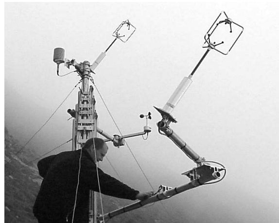
Fig. 3: The setup of the tilted R2 sonics at the slope station Alpe di Gagèrn (2100m).
