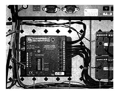
Valves may be controlled by the datalogger via the SDM cable, or manually using the switches on the SDM-CD8S module. The table below indicates which SDM-CD8S channels should be turned on for each sampling system inlet.
