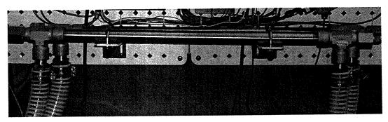
Two more sections of 1" hose connect the dryer purge outlets (labeled "To Pump") to the Busch pump, shown at right.
