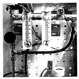
The excess flow from the EC and profile inlets goes through the rotometers mounted at the upper left corner of the sampling system. The 0-25 LPM rotometer on the left carries the EC flow and the 0-10 LPM rotometer on the right carries the profile flow. Note that these rotometers will be at low pressure, so the flow will read higher than the standard flow. At 600 mb they will read approximately 1.3 times the standard flow.
