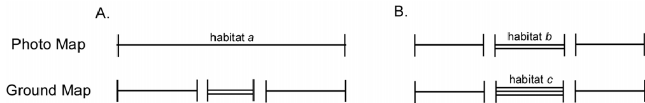
Figure 6. Hypothetical discrepancy in habitat unit counts between the photo-based map and ground-survey map. (A) Habitat type b is missed, a portion of habitat a is mis-identified, and the total count of habitats a and b differs; (B) The count and total length of habitat a are equal between maps and one unit is mis-identified as habitat b rather than habitat c .
