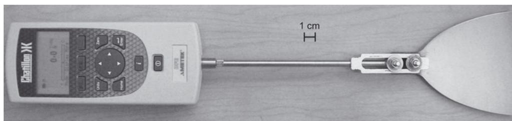
Fig. 3. Blade hardness gauge.
