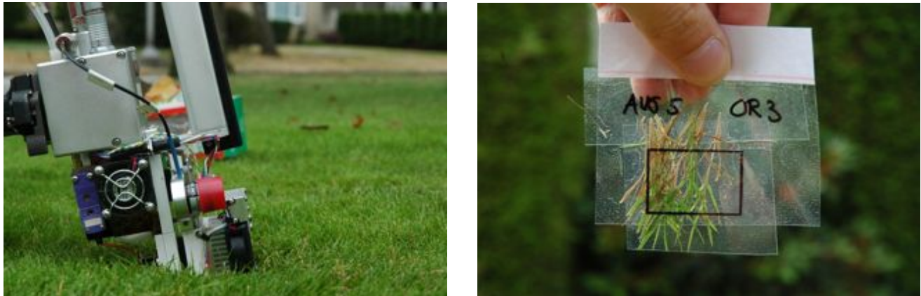
Figure 9 – Li6400 system during measurement of light response curves (left) and subsamples conserved after measurement to estimate leaf area in cuvette (right).
