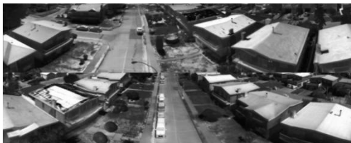
Fig 2. Example of stitched panorama created from thermal images taken at 12:00 PST (south facing at top, north facing below). White represents warmer surfaces.
