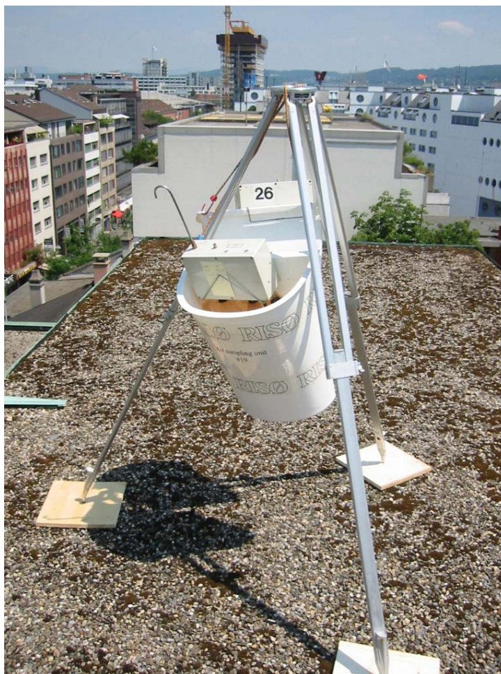
Figure 5 Tracer sampling units during tracer sampling. The two tracer sampling units are attached to a tripod 1.5 m above the roof. The sampling unit is placed at position 8 (see Fig. 2).
