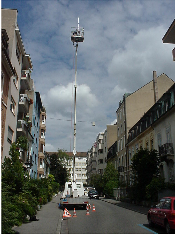
Figure 4 The cherry picker during the tracer release at Florastrasse on 4 July 2002. The release is from the top of the extension that can be seen above the basket of the cherry picker.
